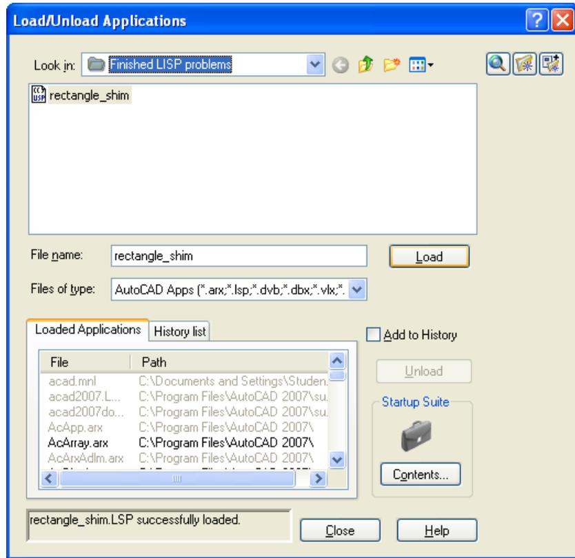
Figure 9.18 – Loading the Rectangle\_shim Program
