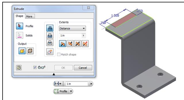
**Figure 5.34 – Select the Extrusion Area**
