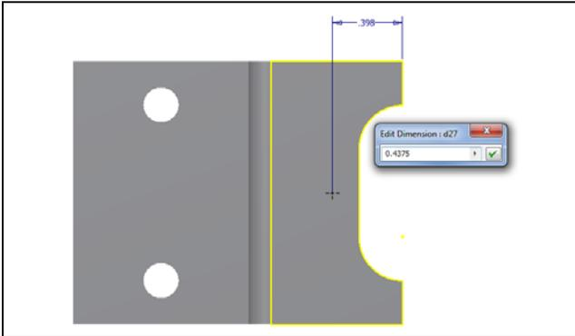
**Figure 5.40 – Dimension the Center Point**
