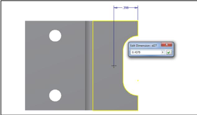
**Figure 5.40 – Dimension the Center Point**
