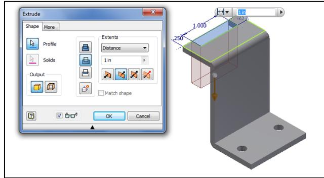
Figure 5.35 – Extrude the Slot
