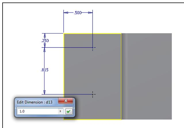
**Figure 5.26 – Dimension the Bottom Center**
