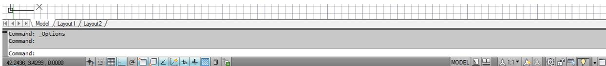
**Figure 2.2 – The command line and the tray**
