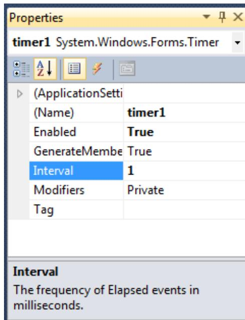
Figure 6A.21 – Setting the Timer's Properties
