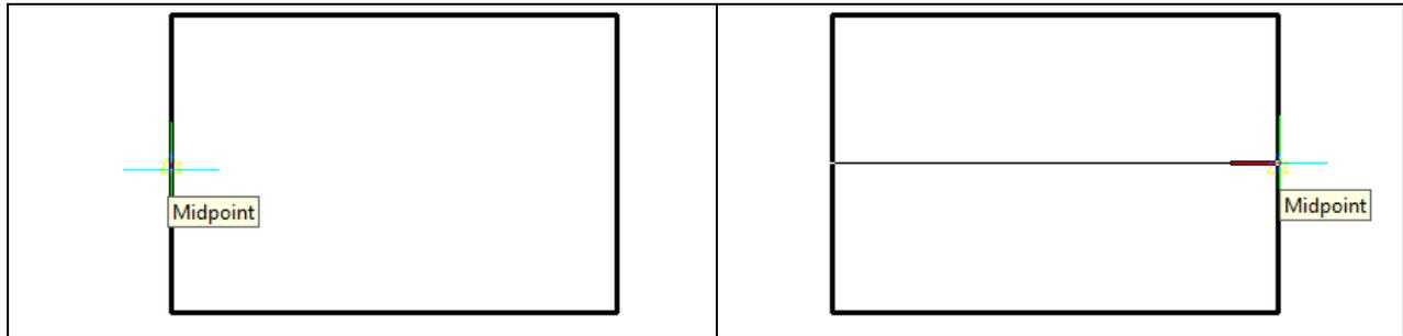
**Figure 1.8 – Selecting the midpoint of a line**      **Figure 1.9 – Selecting another midpoint**
