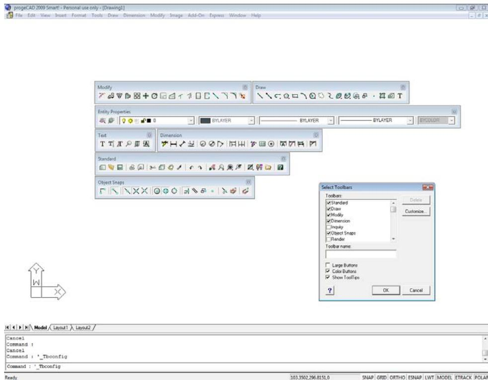
**Figure 1.1** Move the toolbars by placing the mouse pointer over the blue section of the toolbar, clicking and holding the left mouse button and moving the toolbar to the desired position
