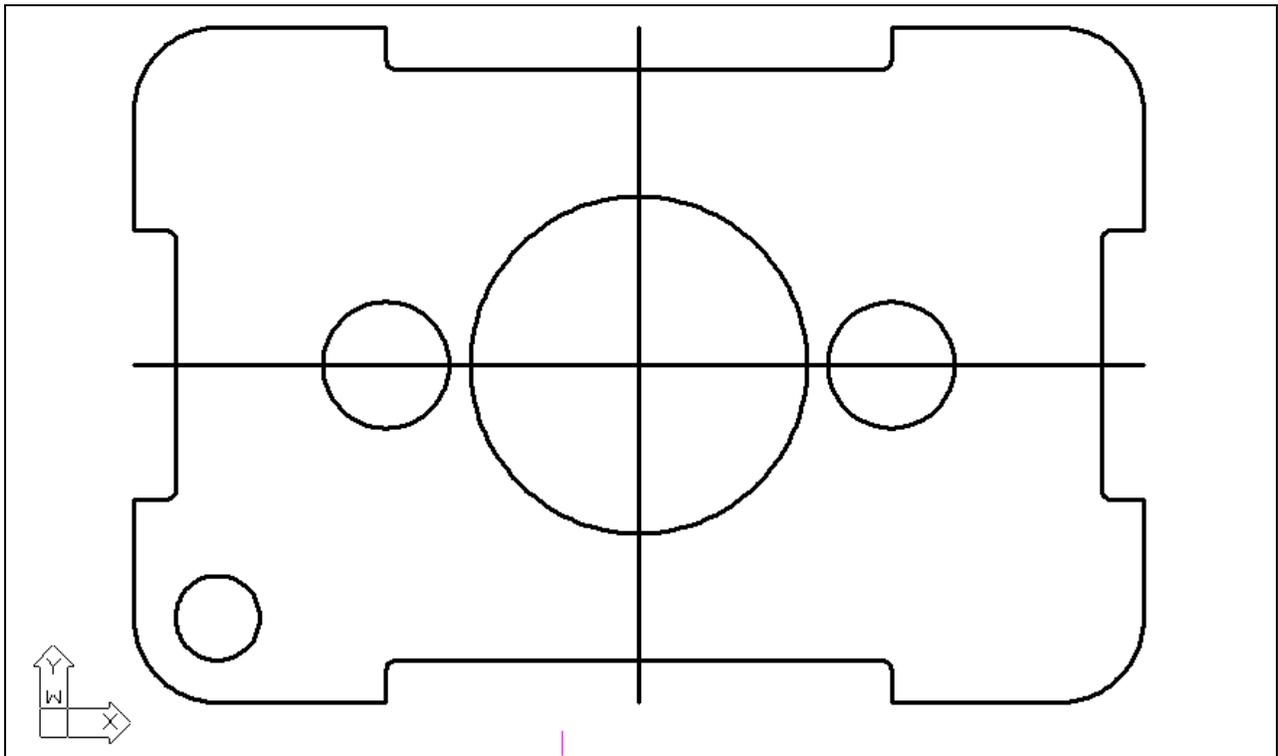
**Figure 2.39 - The Copy command completed, resulting in two circles**
