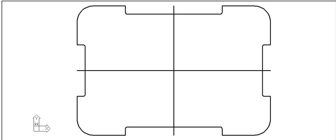
**Figure 1.26** The finished perimeter of your part with two centerlines
