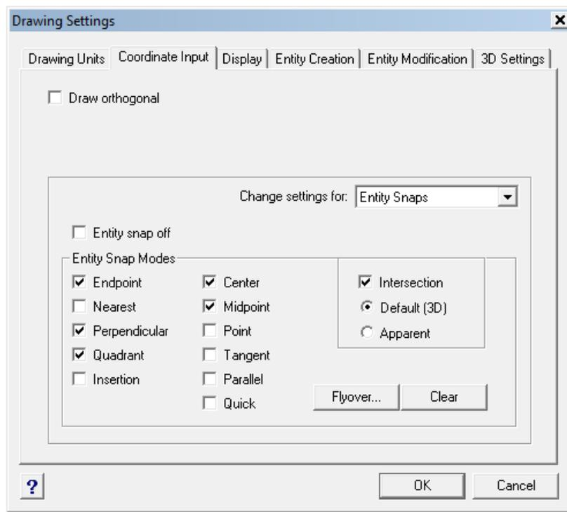
**Figure 1.7 The Entity Snap Settings Area on the Drawing Settings Window**
