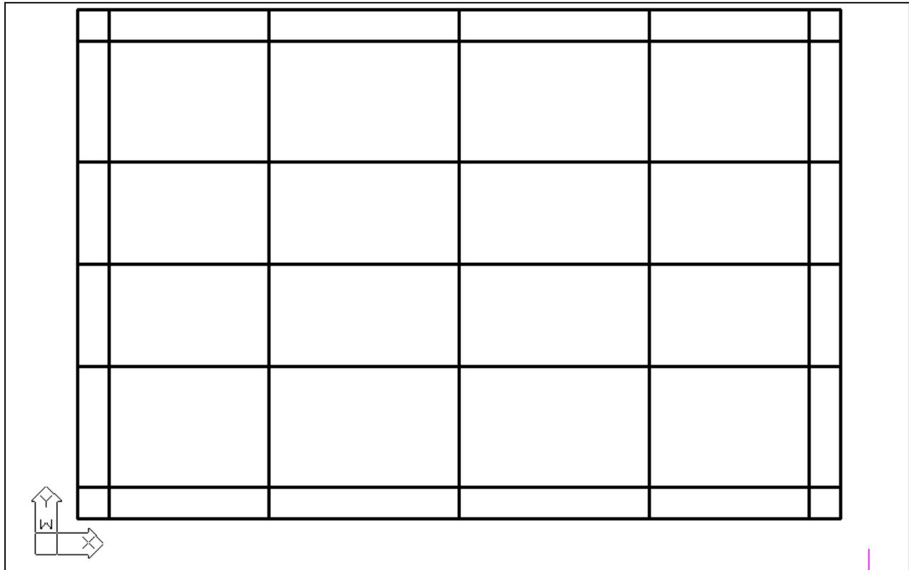
**Figure 1.18** The 4 x 6 rectangle with two centerlines and eight offset lines
