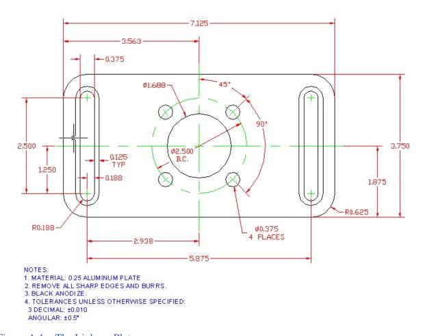
Figure A.1 – The Linkage Plate
