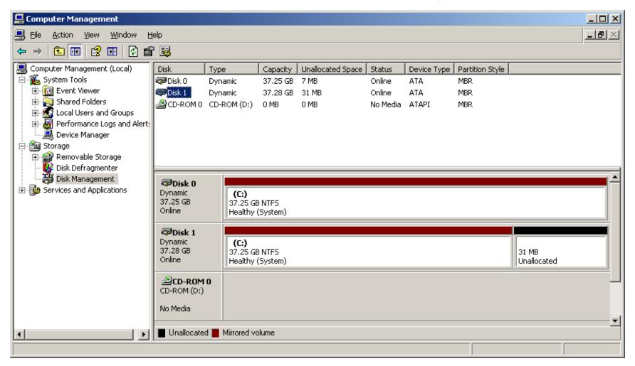
When the drives are synchronized, all data on Drive 0 is copied to Drive 1. The capacity of the server is still only 37.25 GB.
