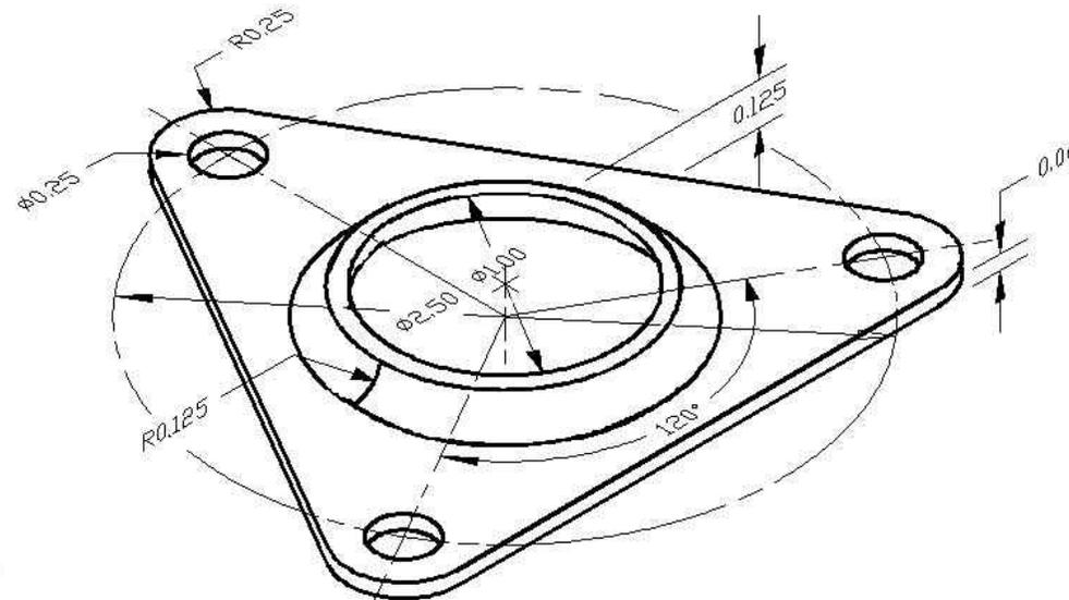
Dimensions are measurements that a factory technician uses to locate a feature or another part. In the sketch shown above, we can see linear and angular dimensions. We can view radiuses and diameters. Whether using orthographic or isometric views, dimensioning and determining tolerance on the measurement is crucial to the design of any product or assembly.
