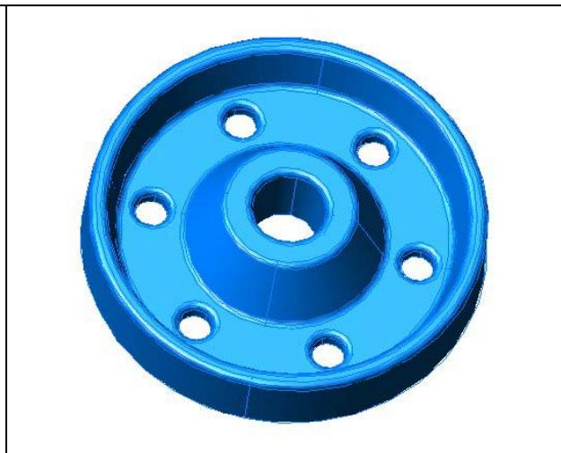
Figure 13.46 – Fillets on the Holes
