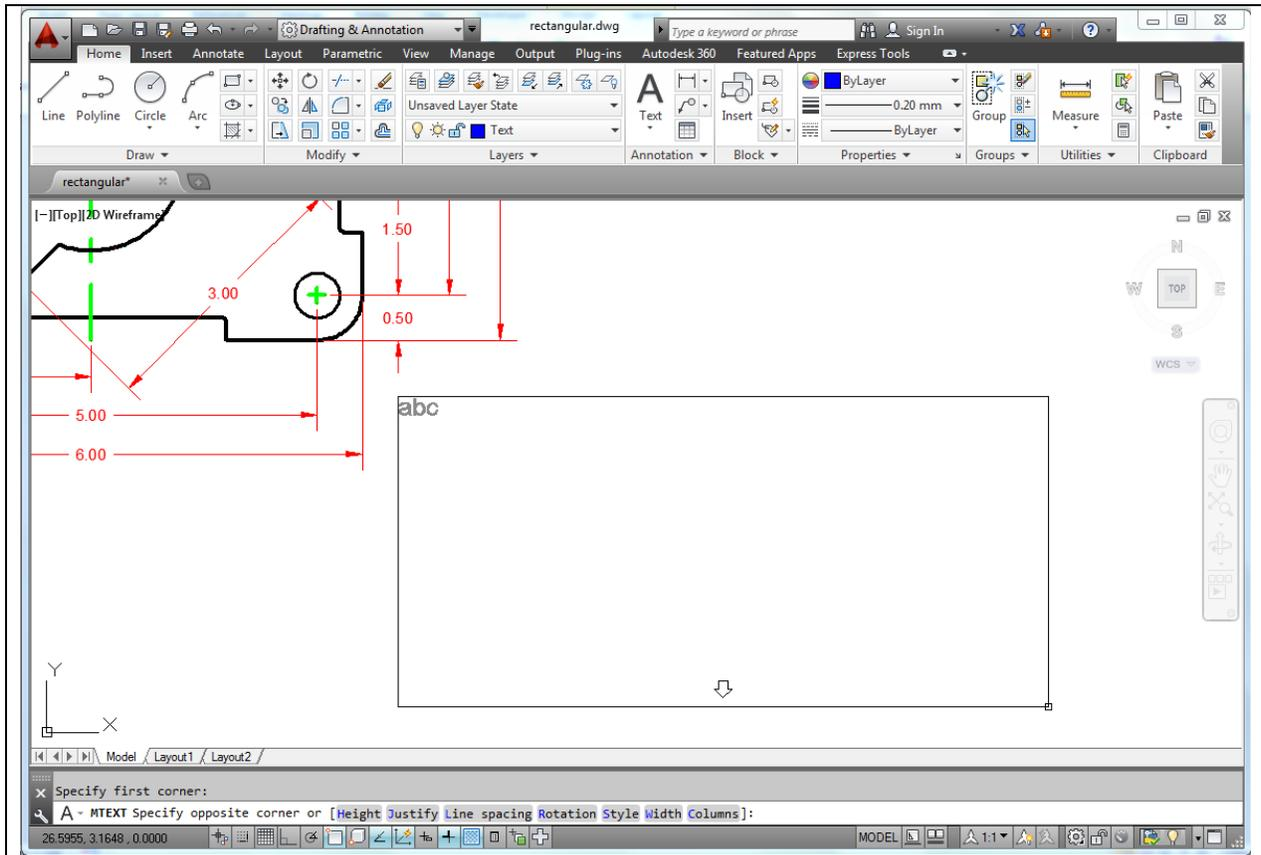
**Figure 4.3 – Making the text window on the drawing**
