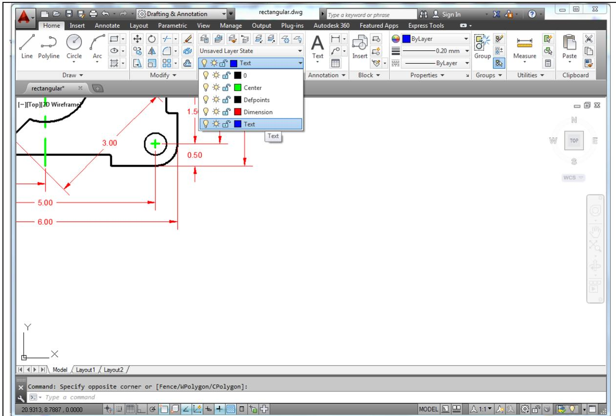
Figure 4.2 – Selecting Text as the active layer
