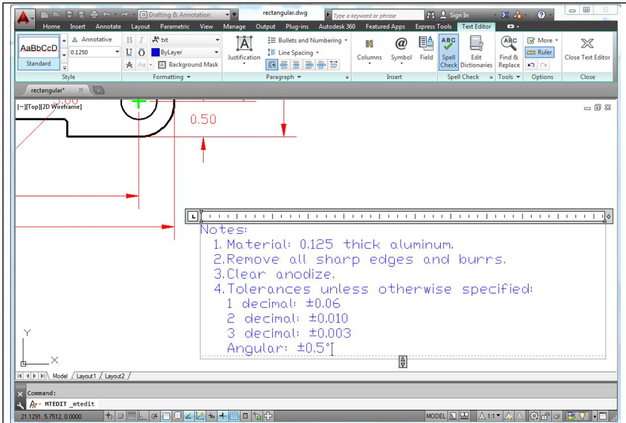
**Figure 4.6 – The finished text**
