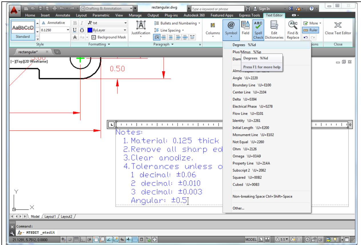
Figure 4.5 – Adding the degrees symbol in the text window
