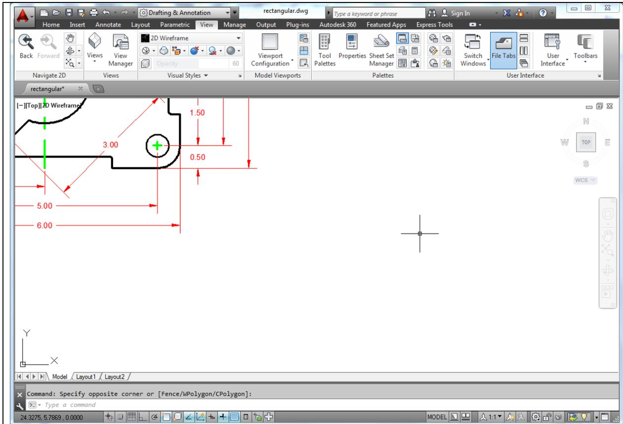
Figure 4.1 – Changing the view in the drawing using the Pan command
