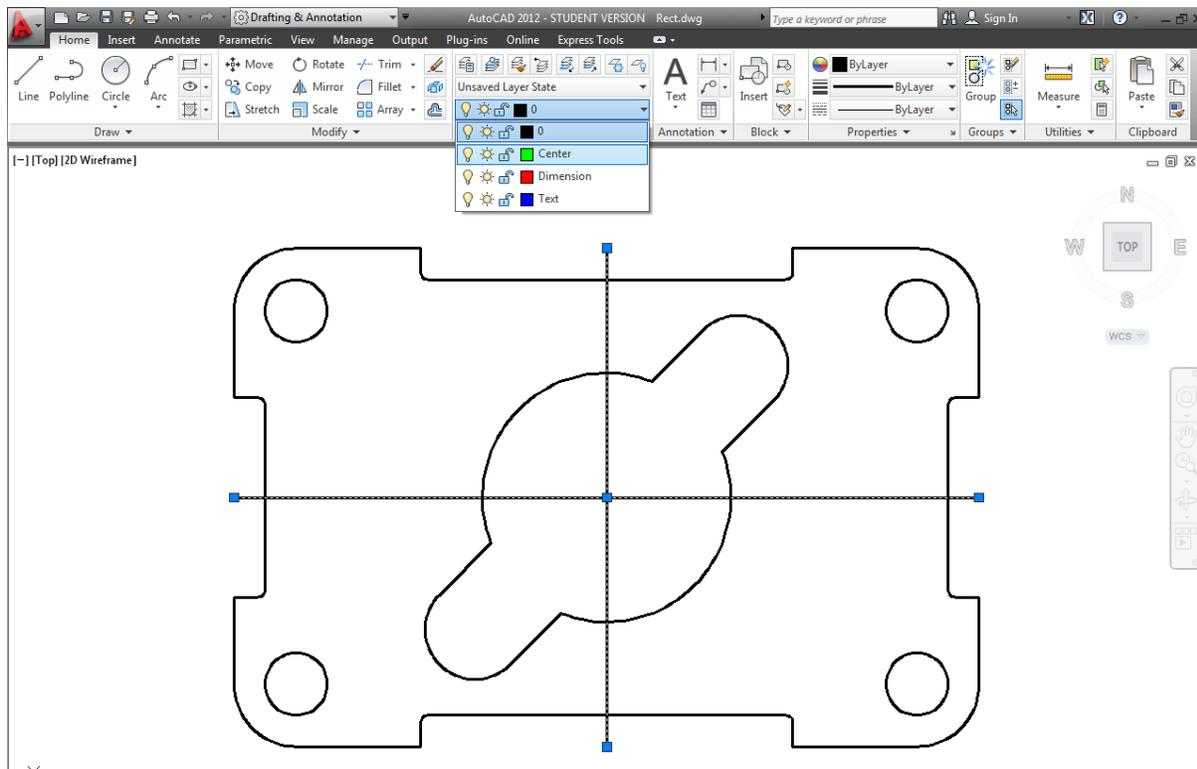
Figure 3.7 – Selecting the Center layer in the Layer Control list box
