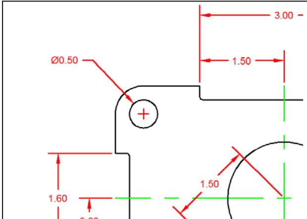
Once again, the aperture cursor will change to a pick box. Select the 0.50 circle located on the upper right hand corner of the part. Similarly to the Radius Dimension command, a second selection will place the diameter text on the drawing (Figure 3.27).
