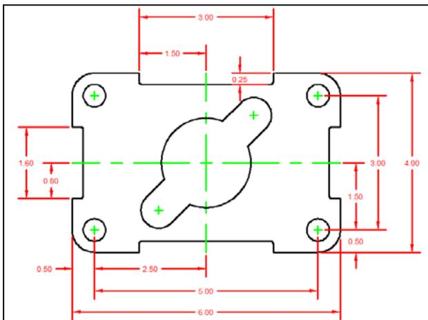
Place the last two dimensions on the left side of the drawing, starting with the 0.80 dimension and then placing the 1.60 dimension. There are 13 linear dimensions on this part.
