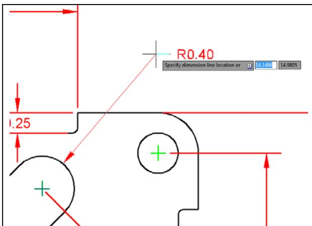
The second radius reinforces the lessons of placing the first radius dimension on the drawing. Again, place the pick box on the 0.40 radius arc (black arc). A second pick of the mouse will place the R0.40 dimension text on the drawing (Figure 3.24).
