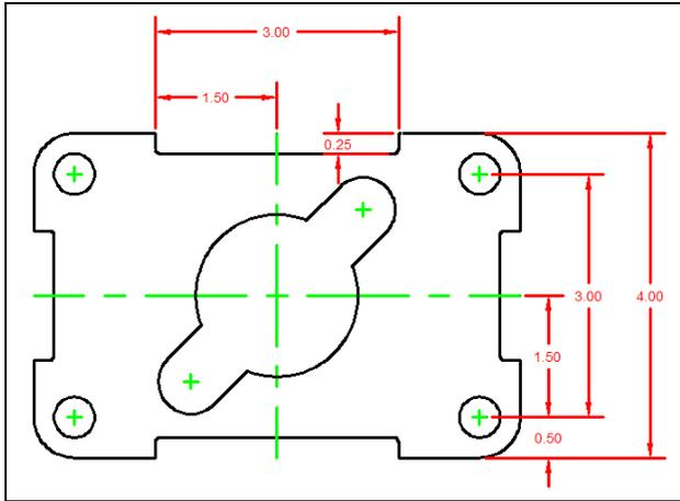
Continue to use the Linear Dimension command by hitting ENTER each time to repeat the command. Always dimension from the inside to the outside of the part so you always have room for more dimensions. Place the 1.50, the 3.00 and 4.00 dimensions, trying to space them evenly (Figure 3.18). To place the 0.50 dimension, start by selecting the right endpoint of the 0.50 centerline. For the third selection to show position, select the 1.50 dimension line. The dimension lines will align.
