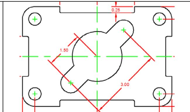
Figure 3.22 – 2<sup>nd</sup> aligned dimension
