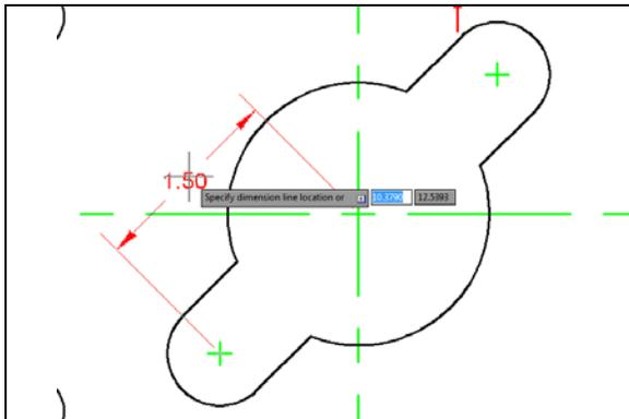
Figure 3.21 – 1<sup>st</sup> aligned dimension
