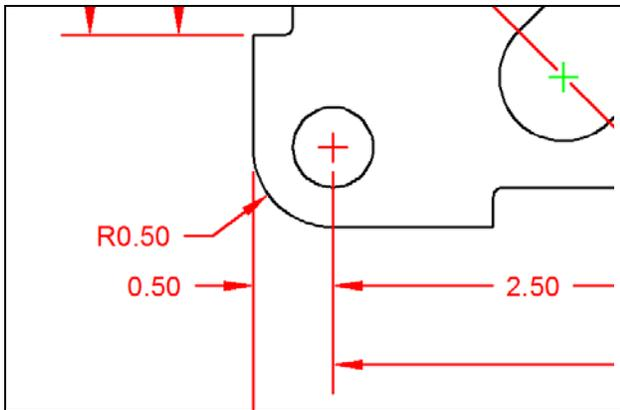
To place a 0.50 radius on the lower left corner of the part, select the Radius Dimension tool on the Dimension toolbar. Place the pick box on the 0.50 radius arc (black arc). A second pick of the mouse will place the R0.50 dimension text on the drawing. Notice that moving your mouse around the circumference of the center point will change the location of where the pointing arrow intersects with the arc. A red center mark is placed on the drawing with the radius dimension (Figure 3.23).
