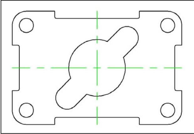
The Center layer now replaces the 0 layer in the Layer list box to show that these two lines now reside on the Center layer. Press the ESC key on your keyboard and the lines are no longer dotted and are removed from the selection set. Centerlines are critical in the dimensioning process since they show symmetry in a part and reduce the amount of dimensions on the drawing.
