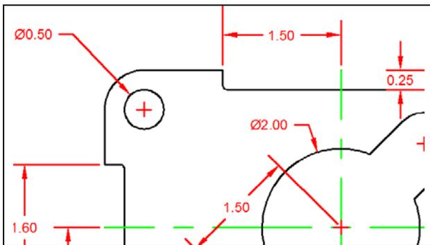
The second diameter you will place on the drawing is on the 2.00 diameter hole in the center of the part. Select the Diameter Dimension tool on the Dimension toolbar and the aperture cursor will change to a pick box. Select the 2.00 circle. Make your second selection to place the dimension text on the drawing (Figure 3.28).
